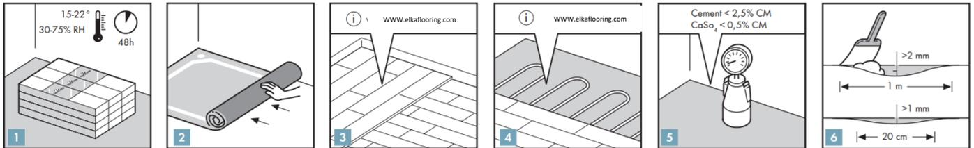
Let the planks acclimatize for 48 hours in the unopened packaging at the normal room temperature, in the middle of the room where the floor is to be installed. The ideal conditions are 15-22°C at a relative humidity of 30-75%. If climate conditions are outside this 30-75% range, we strongly advise to acclimatize for 1 week with opened packages.
